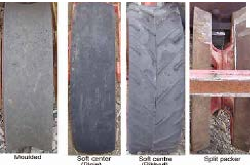
Figure 125: Typical over-centre press wheel profiles
